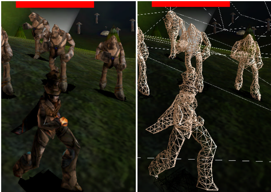
Figure 1. Note the smooth, rounded nature of the characters in this shot from Sacrifice . The smoothness is made possible by the high polygon count, as seen in the right hand image.
