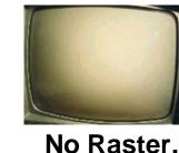
(No light being produced on the CRT face plate)
