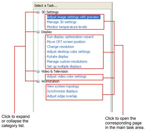
Figure 3.3 NVIDIA Control Panel Select a Task pane
